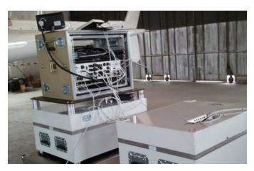
**AGRS SYSTEM** with 33.6 litres of sensor and equipment rack ready for installation in aircraft
